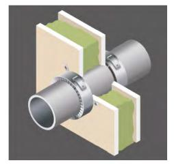
**Wall Penetrations:** FP170 should typically be fixed on both sides of any suitable wall construction
