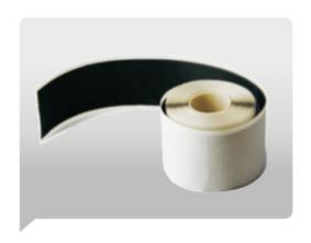
TREMproof FBM Sealed Tape is specially formulated double sided, reinforced pressure sensitive tape. The tape has two layers of pressure sensitive adhesive which bond respectively to the sand and HDPE surface. The specially developed adhesive layers work together to form a continuous and integral seal to the structure. The structure of TREMproof FBM Sealed Tape is as follow:
